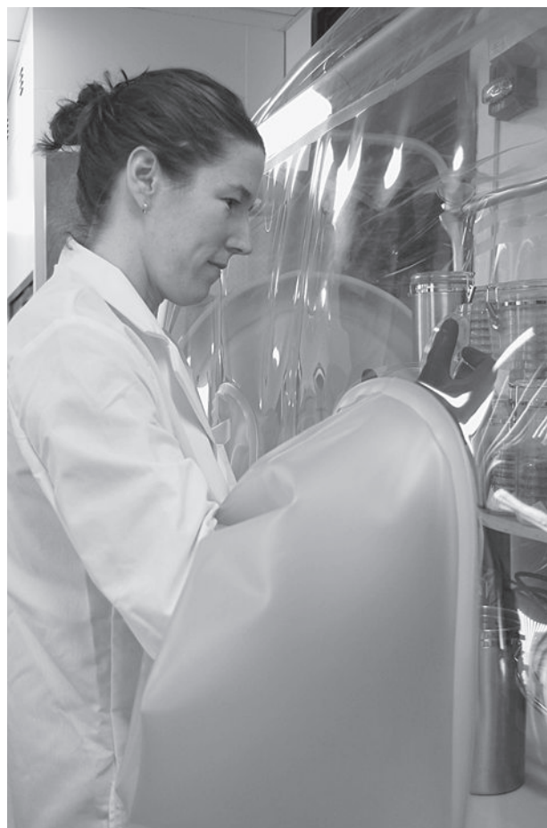
Anaerobic chambers allow microbiologists to work with cultures in an oxygen-free atmosphere. ( Geobacter Project, University of Massachusetts, Amherst)
