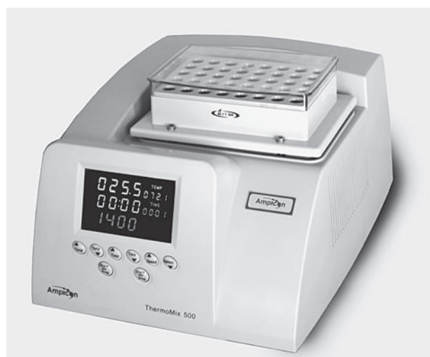
Thermocyclers raise and lower incubation temperatures to automate the polymerase chain reaction (PCR). (PCRStation)
